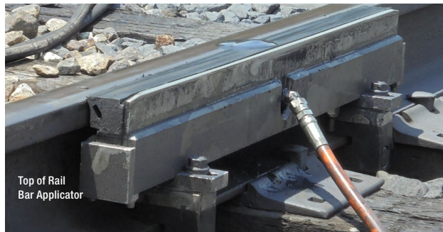
Gauge Face Applicator Bar Three Component Assembly
